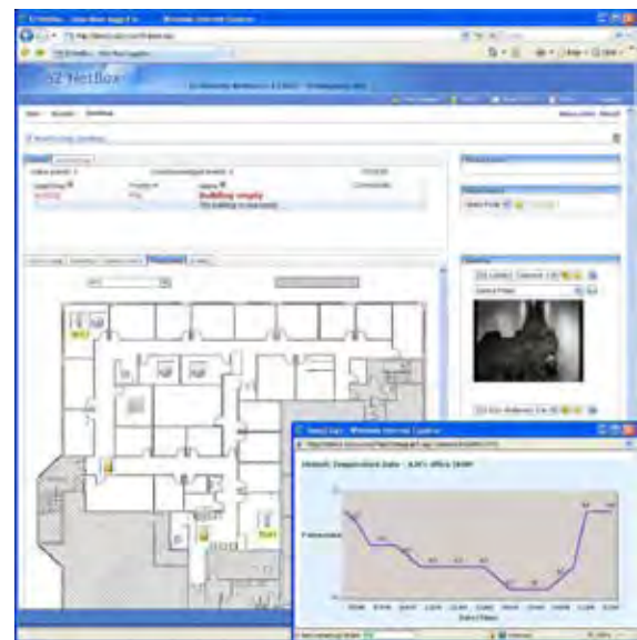
Dynamic floorplan graphics show event and status data in real time. This example also shows temperature trend charting.
